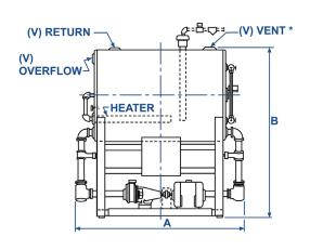
\* Connect unobstructed full size vent to atmosphere. Do not valve or plug.
