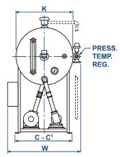
Note: 60 gallon duplex units. One pump will be mounted outside. Dim  $C^1$
